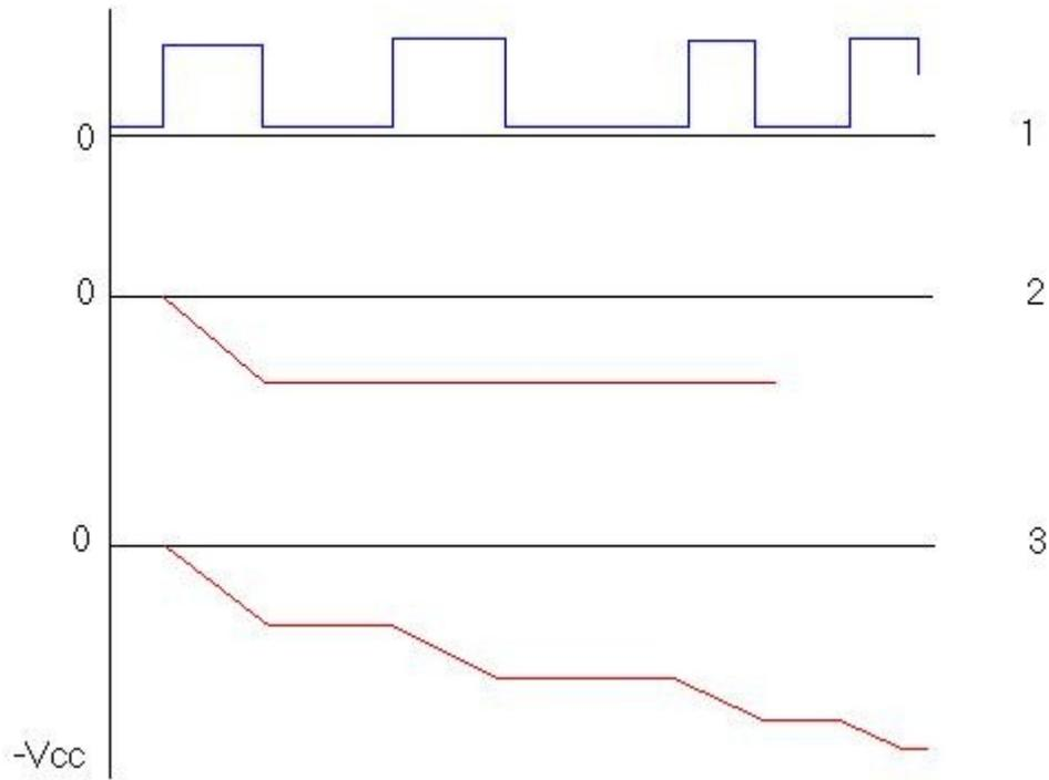
**Q5.** In the above circuit (Ref Q4), let  $R = 10\text{K}\Omega$   $C = 10\text{nF}$ . If the integrator capacitor is shunted by a  $1\text{M}\Omega$  resistor, how will be the response for an input pulse of 1-V height and 1ms width?
