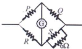
$$\frac{P}{Q} = \frac{R}{S \parallel (S+6)}; P = Q = R = 2\Omega; \Rightarrow S = 3\Omega$$
